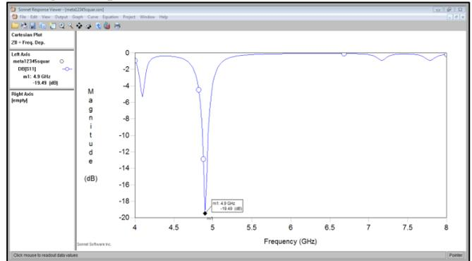
Fig. 4: depicts the return loss (S<sub>11</sub>) characteristics of unloaded rectangular slotted microstrip patch
