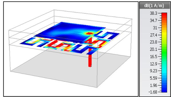
Fig. 8: Surface current distribution (A/m)
