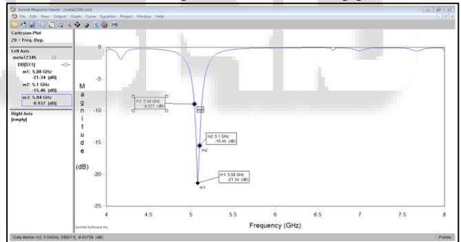
Fig. 5: depicts the return loss (S<sub>11</sub>) characteristics of unloaded rectangular slotted microstrip patch
