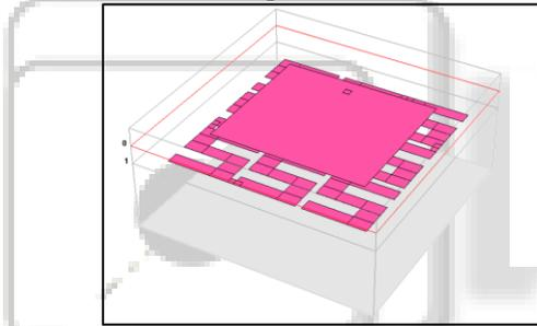
Fig. 2 Rectangular microstrip patch antenna with microstrip feed line
