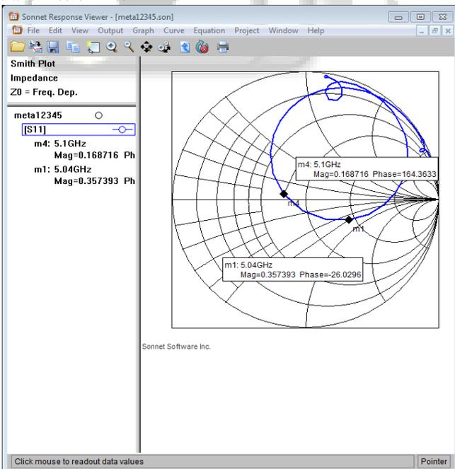
Fig. 7: Smith chart of the triangular metamaterial antenna
