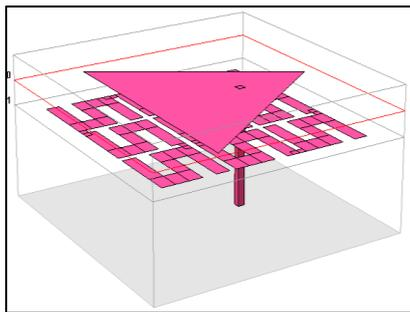
Fig. 3: Triangular microstrip patch antenna with microstrip feed line
