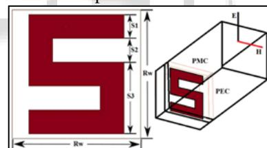
Fig. 1: Top view, of S-shape unit cell, a view of boundary conditions for EM analysis of S-RIS unit cell.
