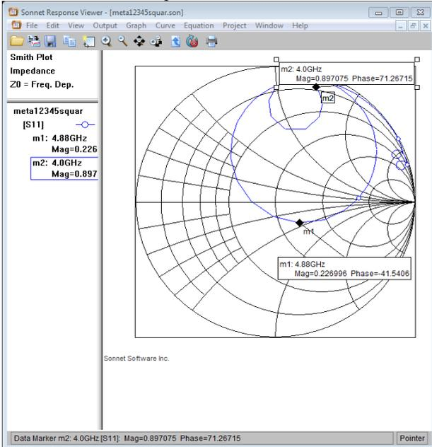
Fig. 6: Smith chart of the square metamaterial antenna
