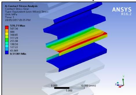
Fig. 1: Contact stress of involute gear
