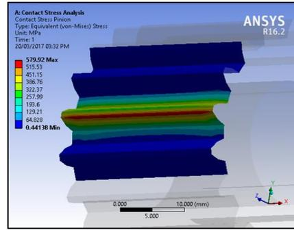
Fig. 3: Contact stress of involute pinion
