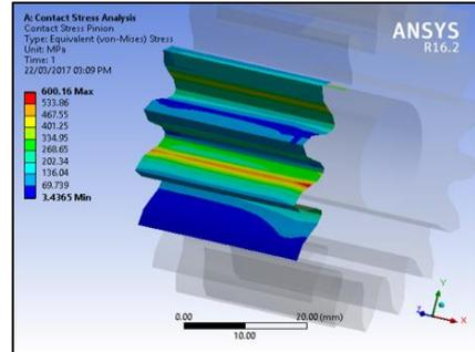
Fig. 4: Contact stress of cycloid pinion
