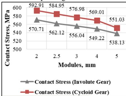
Fig. 7: Variation of contact stress for different modules in involute and cycloid gear teeth
