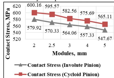
Fig. 5: Variation of contact stress for different modules for involute and cycloid pinion teeth
