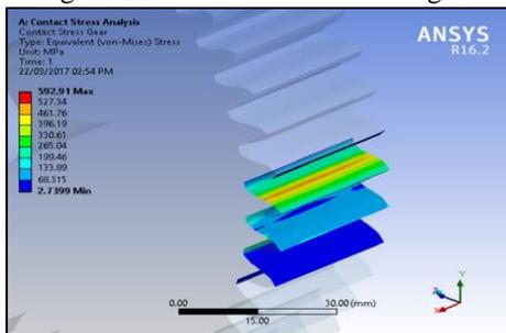
Fig. 2: Contact stress of cycloidal gear
