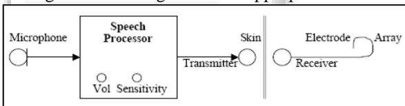
Fig 5. : Components of cochlear implant system image courtesy of Cochlear Ltd
