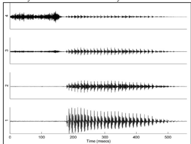
Fig. 9: Bandpassed waveforms of the syllable "sa" produced by a simplified implementation of the compressed analogue approach.
