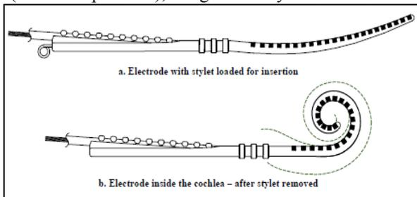
Fig 7: Pre-curved electrode array(a) Electrode with stylet loaded for insertion (b)Electrode inside the cochlea-after stylet removed image courtesy of Cochlear Ltd.
