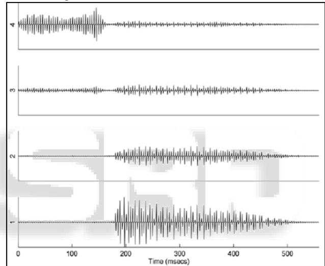
Fig. 12: Pulsatile waveforms of the syllable “sa” produced by a simplified implementation of the CIS strategy using a four-channel implant. The pulse amplitudes reflect the envelopes of the bandpass outputs for each channel. The pulsatile waveforms are shown prior to compression.
