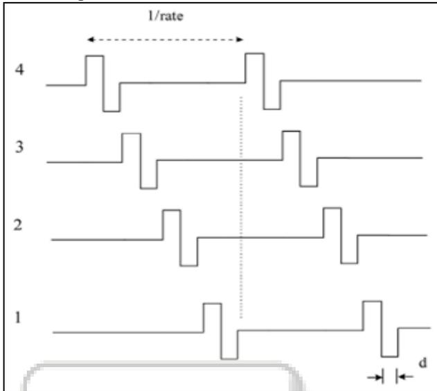
Fig. 10: Continuous Interleaved Sampling (CIS) Approach.
