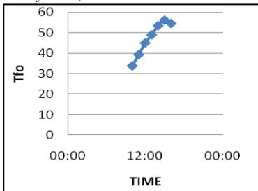
Fig. 7: Time Vs Collector outlet (Tfo)
