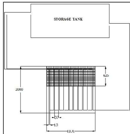
Fig. 2: Upper half covered glazed and unglazed PV/T collector.
