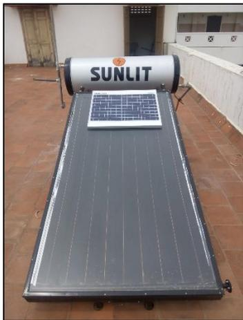
Fig. 12: Upper half covered PV/T Collector
