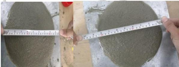
Fig. 1: Flow Test of C90E6S4
