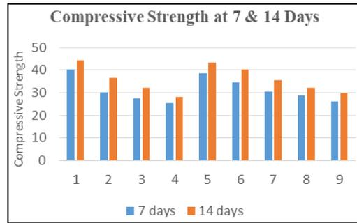
Fig. 2: Graphically represents the Compressive Strength of egg shell concrete Cubes.
