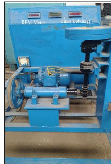
Fig. 1: Disc on disc type of rolling wear analysis machine
