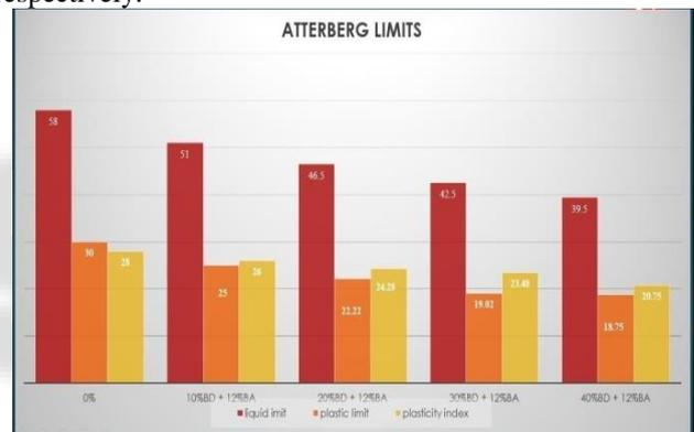
Fig. 4: Comparison of atterberg's limit
