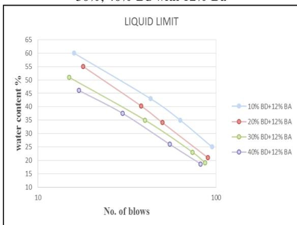
Fig. 3: Liquid limit curve for various proportion of BD
