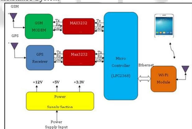
Fig. 1: Block diagram of PDSA system
