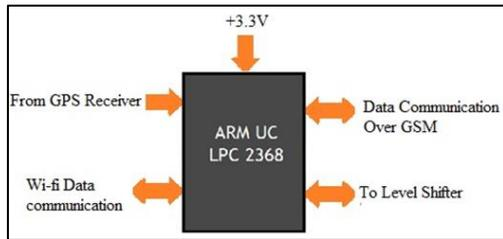
Fig. 2: Microcontroller and Interfaces
