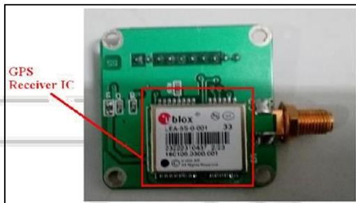
Fig. 3: GPS receiver Module
