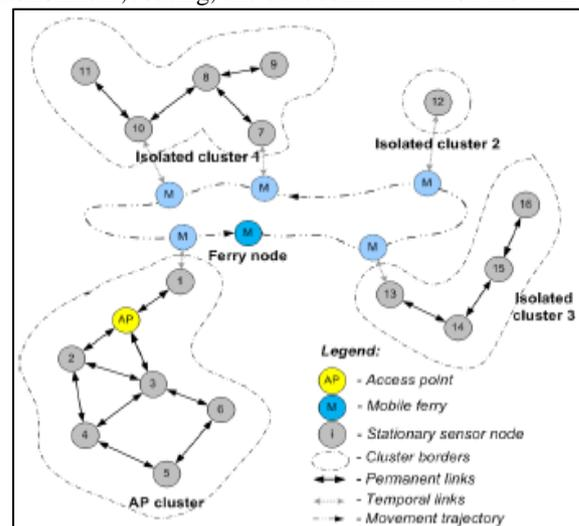
Fig. 1: Example of the WSN with Mobile Ferries.
