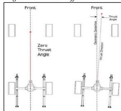
Fig. 17: Thrust Angle/ Wheel Base Difference
