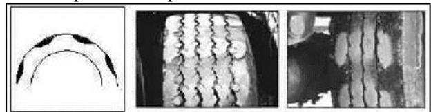
Fig. 13: Cupping/Scallop Wear
