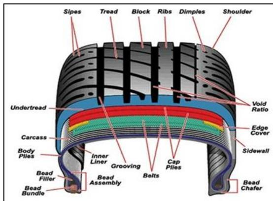
Fig. 1: Structure of tyre
