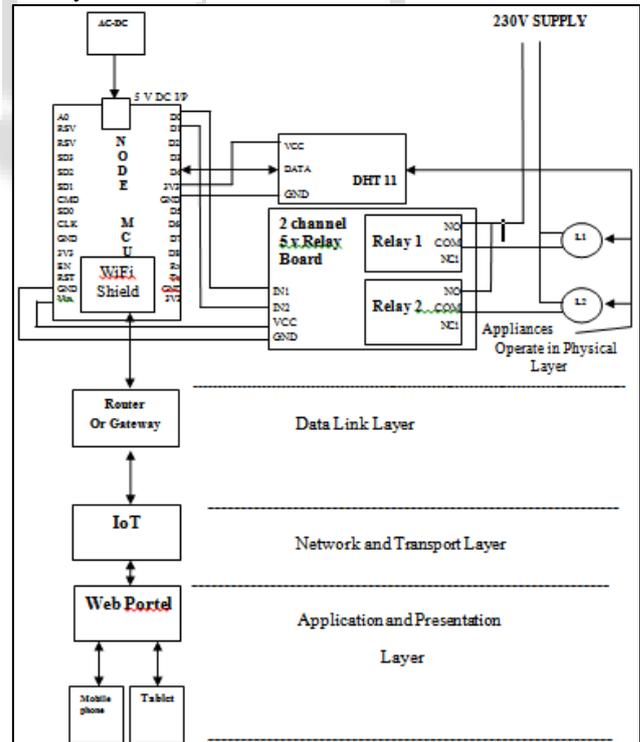
Fig. 4: General block diagram of smart homes circuit through IoT
