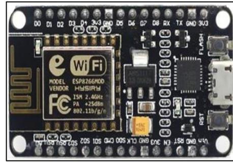
Fig. 2: Node MCU ESP8266 12E
