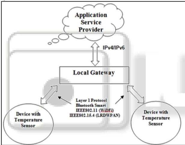
Fig. 1: Device-to-gateway communication model diagram.
