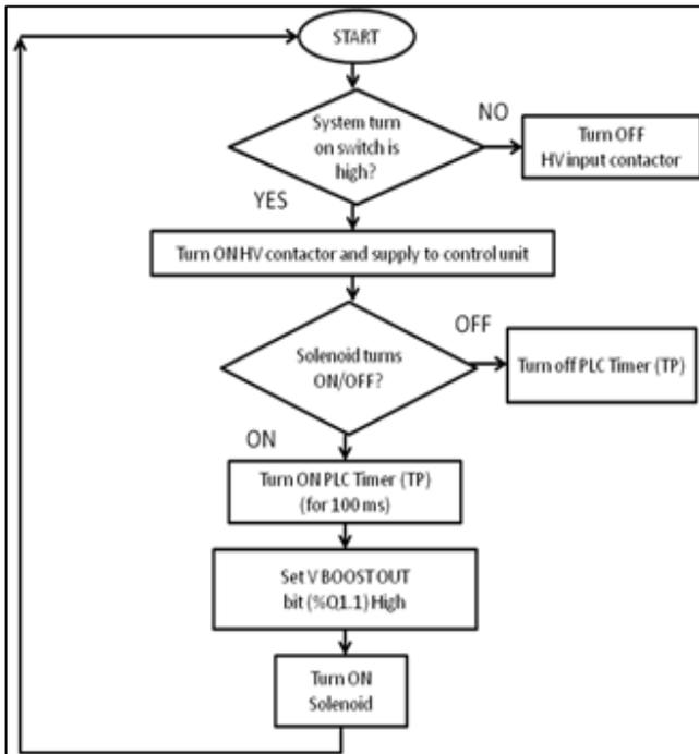
Fig. 4: Flow chart of operation of solenoids using PLC.
