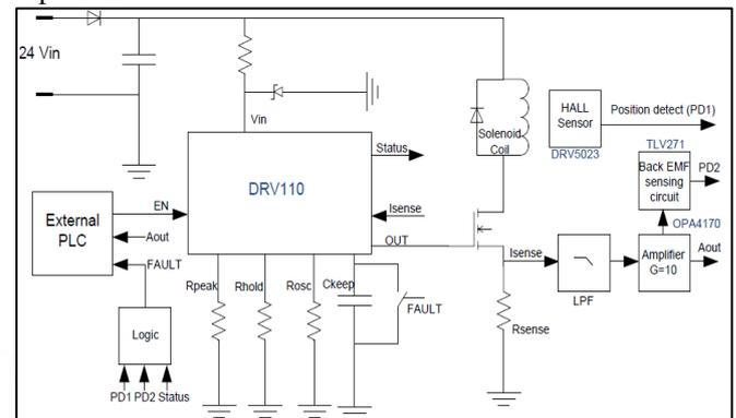
Fig. 1: Block diagram of solenoid driver using DRV110.
