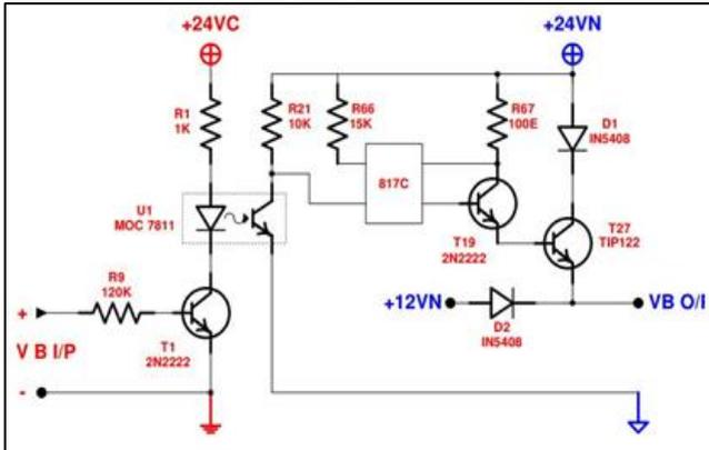
Fig. 3: Voltage-booster circuit using PLC.
