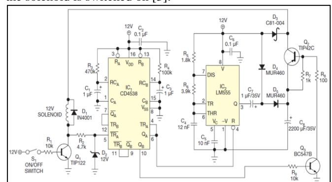
Fig. 2: Voltage-booster circuit to drive a solenoid rated at a 12 V DC supply voltage.
