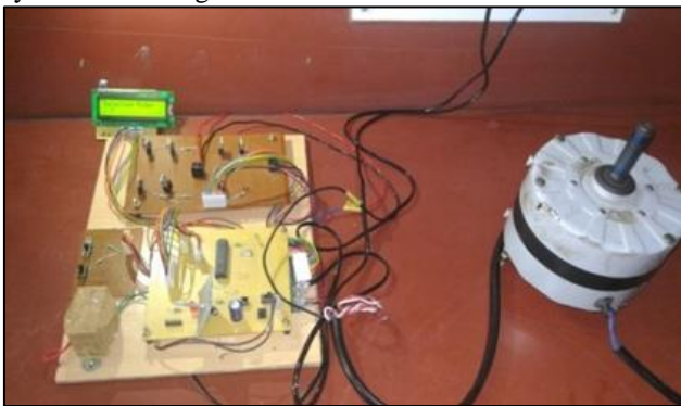
Fig. 3: Hardware model of cycloconverter with induction motor.
