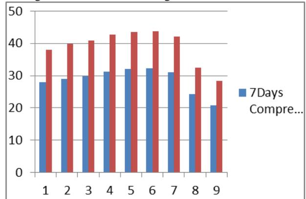
Graph 5, 7 & 28 -Days concrete Compressive Strength vs. Replacement of Coarse and fine aggregates by Steel slag and Waste glass Powder
