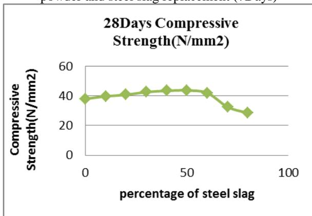
Graph 4: Compressive Strength of cubes for combined glass powder and steel slag replacement (28Days)
