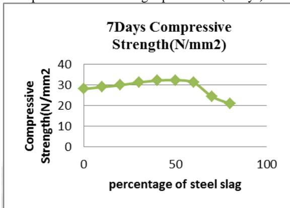
Graph 3: Compressive Strength of cubes for combined glass powder and steel slag replacement(7Days)
