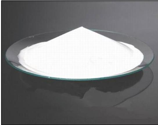
Fig. 1: Crushed Waste Glass
