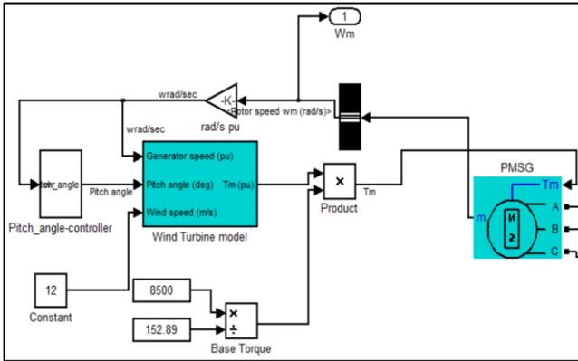
Fig. 4: Wind Turbine linked with Synchronous Generator
