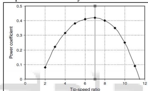
Fig. 2: Power Coefficient vs. Tip-Speed Ratio
