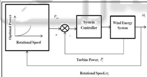
Fig. 1: Power Signal Feedback Method
