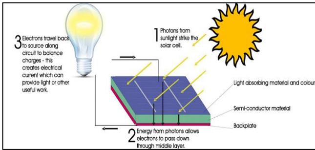
Fig. 1.2: Working of photovoltaic panels
