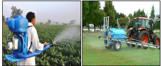
Fig. 1.1: Portable sprayer and Trailed sprayer
