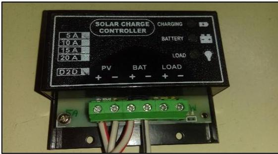
Fig. 4.3: Solar charge controller
