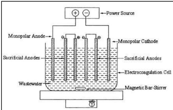
Fig. 1: Bench-scale EC reactor with Monopolar electrodes in serial connection.
