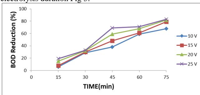
Fig. 3: BOD removal with electrolysis time for different voltages at pH 7.0
