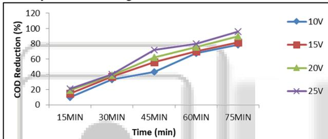
Fig. 2: COD removal with electrolysis time for different voltages at pH 7.0
