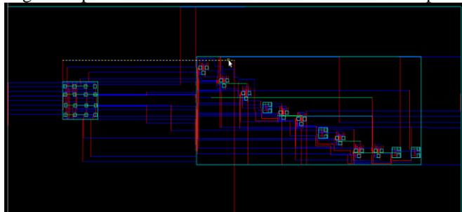
Fig. 10: Layout of 4 bit Wallace Multiplier
