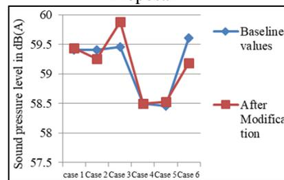
Fig. 9: Comparison between sound pressure levels of base model of blower & modified model of blower
