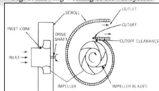
Fig. 2: Schematic of main parts of centrifugal fan
