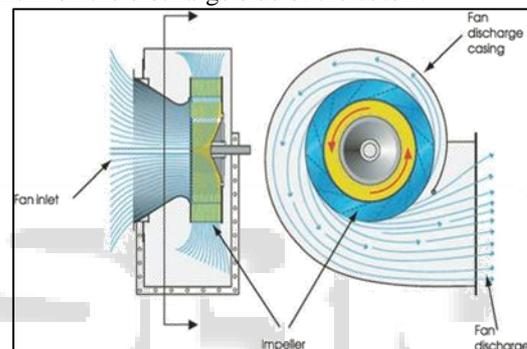
Fig. 1: showing working of blower system
