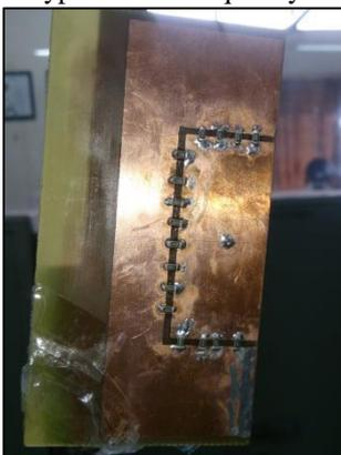
Fig. 17: Prototype of dual frequency PIF antenna
