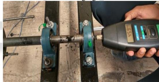
Fig. 3: Measure the speed of shaft with tachometer
