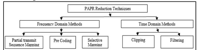
Fig. 2: Classification of PAPR reduction methods
