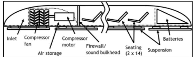
Fig. 3: Hyperloop passenger capsule subsystem national locations (not to scale)
