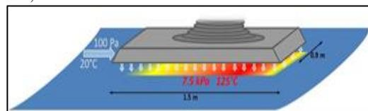
Fig. 7: Schematic of air bearing skis that support the capsule.
