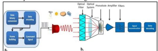
Fig. 1: Architecture of a VLC system: a. Emitter; b. Receiver
