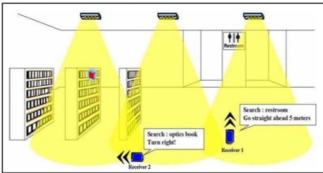
Fig. 5: VLC usage for indoor localization
