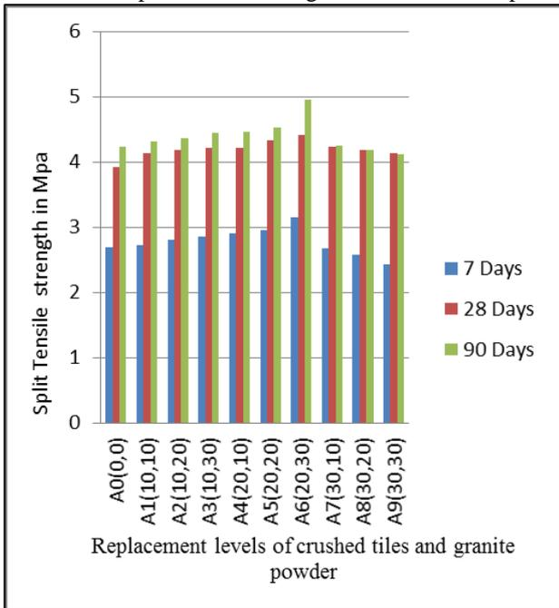
Fig. 5: Split Tensile strength of concrete In Normal Water Curing
