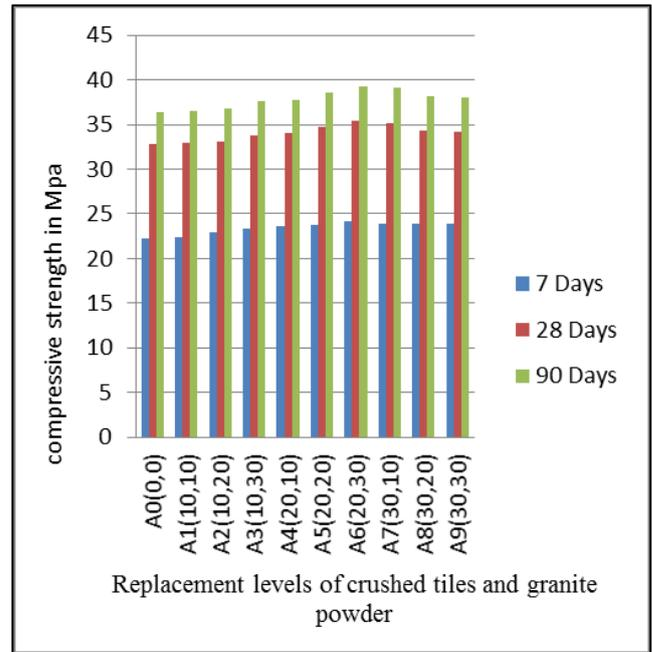
Fig. 4: Compressive strength of concrete In Accelerated Curing Tank.
