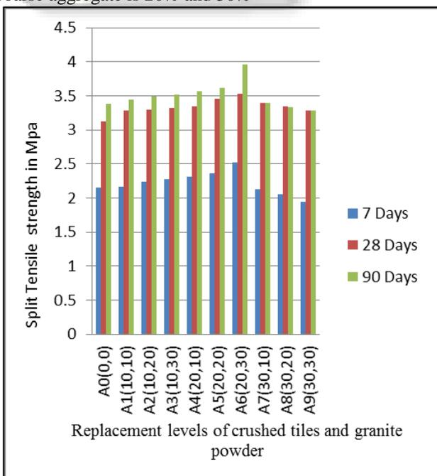
Fig. 6: Split Tensile strength of concrete In Accelerated Curing Tank
