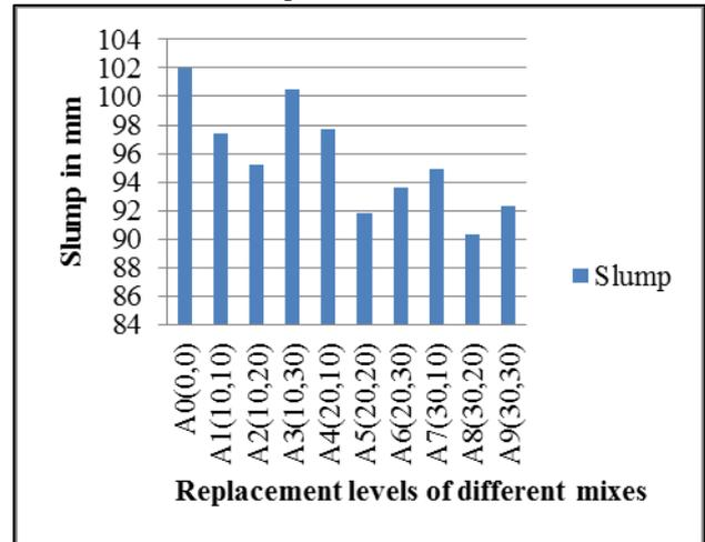
Fig. 1: slump test results
