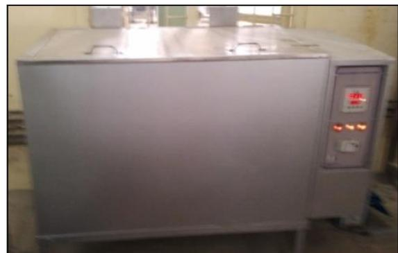
Fig. 2: Accelerated curing tank
