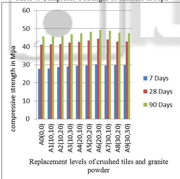
Fig. 3: Compressive strength of concrete In Normal Water Curing
