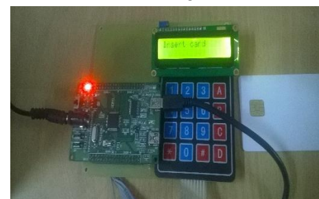
Fig. 6: Photo 4 Hardware Module (Smart Card is to be inserted)
