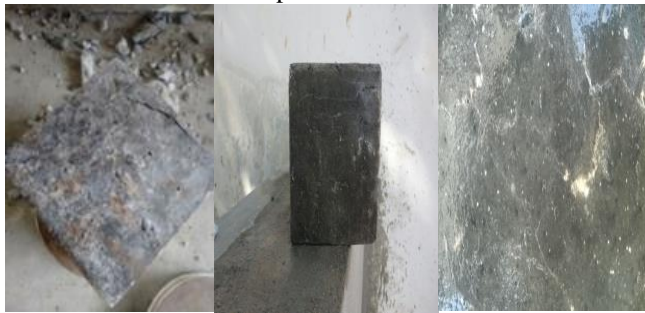
Fig. 2: The self healing behaviour in high percentage bacteria ( 20gm ) is shown in above figures.
