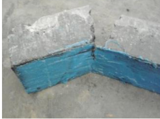
Fig. 2: Failure of Beam with CFRP on tension side of dimension 500*100*10mm.
