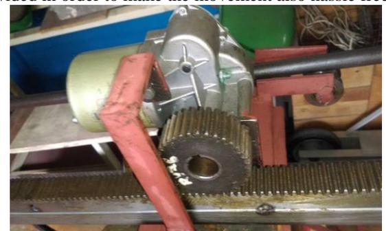
Fig. 5: Rack and Pinion For X Axis Movement
