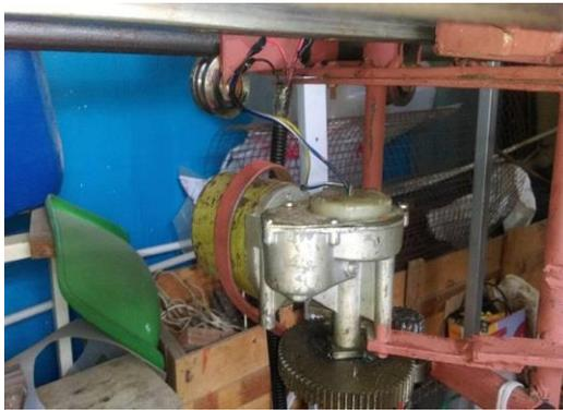
Fig. 6: Pair of Spur Gears for Upward Movement
