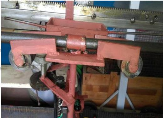
Fig. 7: Carriage Assembly for Brushes
