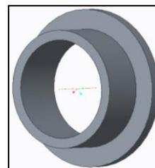
Fig. 1: Isometric view of Bush
