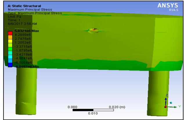
Fig. 4: Stress Distribution on Mould
