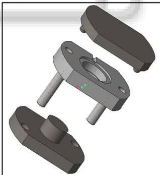
Fig. 3: Exploded View of Mould
