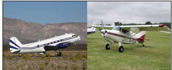
Fig. 1.1: Tail wheel configuration landing gear on a DC-3 (left) & Super Rocket
