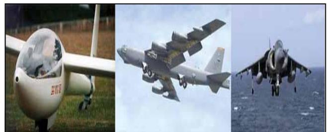
Fig. 1.2: Tandem landing gear along the longitudinal axis of the aircraft permits the use of flexible wings on sailplanes (left) and select military aircraft like the B-52 (centre). The VTOL Harrier (right) has tandem gear with outrigger-type gear.
