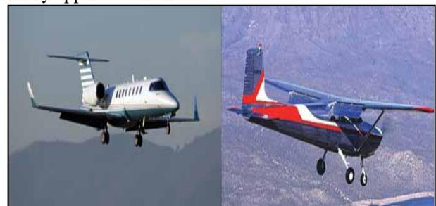
Fig. 1.3: Tricycle-type landing gear with dual main wheels on a Lear jet (left) and a Cessna 172, also with tricycle gear (right).
