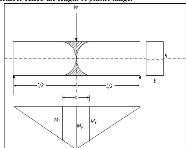
Fig. 5: Hinged Length of a Simply Supported Beam with Central Concentrated Load
