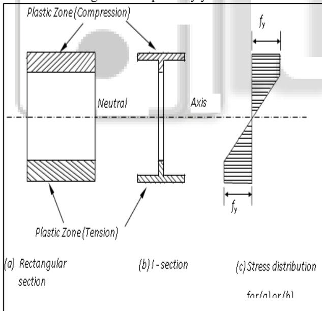
Fig. 3: Stresses in Partially Plastic Beams
