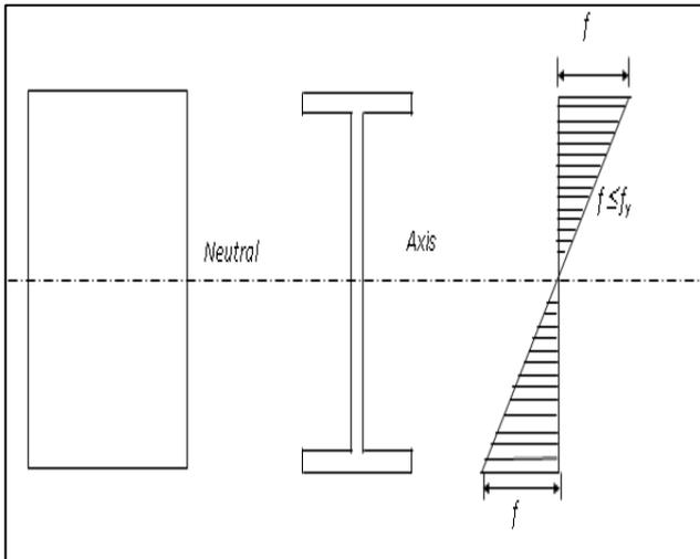
Fig. 2: Elastic Stresses in Beams
