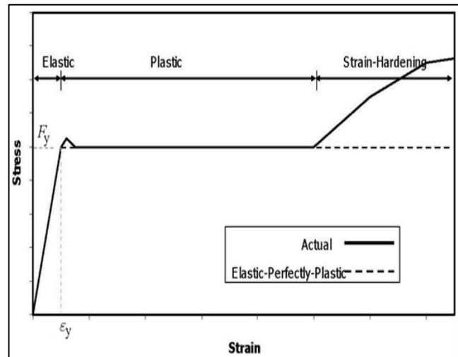
Fig. 1: Typical Stress-Strain Diagram of Structural Steel.
