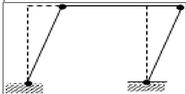
Fig. 8: Panel or Sway Mechanism
