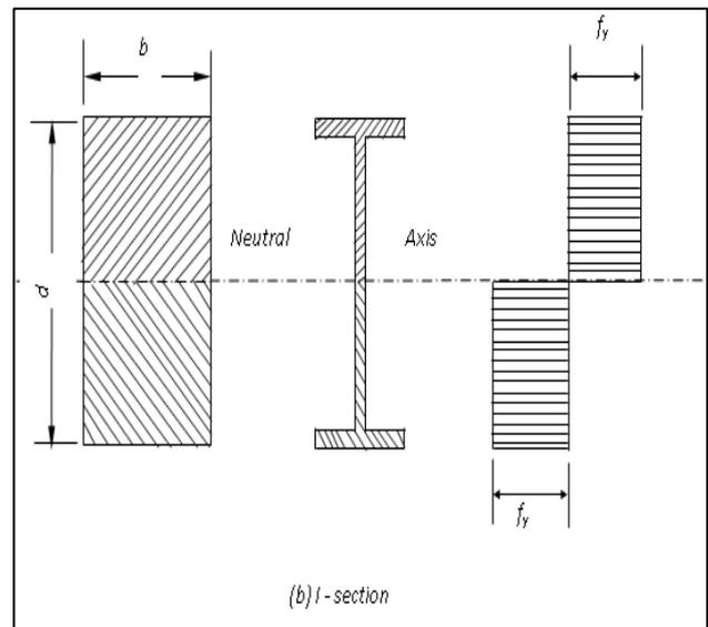
Fig. 4: Stresses in Fully Plastic Beams
