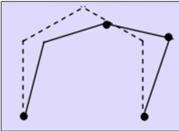
Fig. 9: Gable Mechanism
