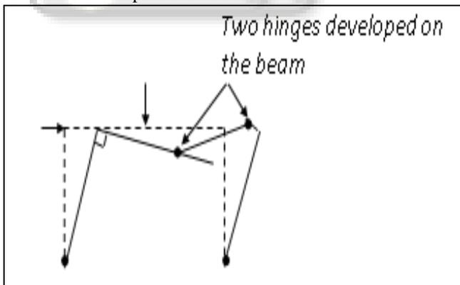
Fig. 11: Combined Mechanism
