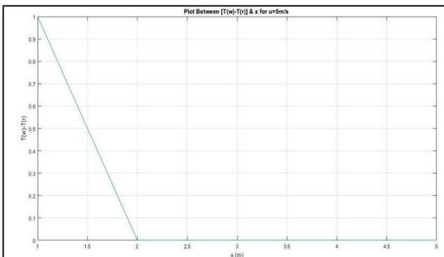
Fig. 3: Graph between instantaneous temperature difference and position in the regenerator at any air velocity of 5 m/s
