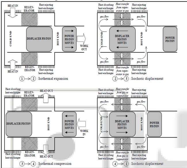
Fig. 2: Thermodynamic processes in the ideal Stirling-cycle refrigerator/heat-pump as shown on a simplified Beta-configuration machine.
