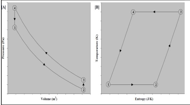
Fig. 1: Pressure-volume and temperature-entropy process diagram of Stirling Refrigerator
