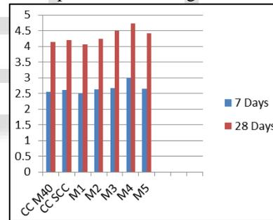
Fig. 2: Split Tensile Strength Test Results
