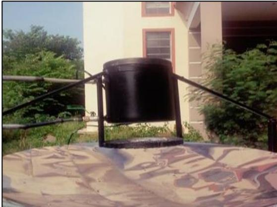
Fig.2: Oil Receiver Tank
