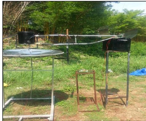
Fig. 8: Fabricated Energy Stored Sensible Hybrid Solar Cooker
