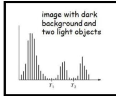
Fig. 4(a): Showing threshold graph of an image with dark background and two light objects
