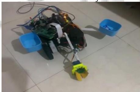
Fig. 4.1: Detecting and Picking the object
