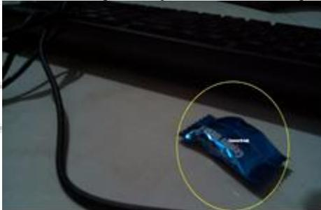
Fig. 3.4: Encircling the detected object to get coordinates of the center of the object.
