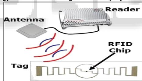
Fig. 4: Basic RFID system
