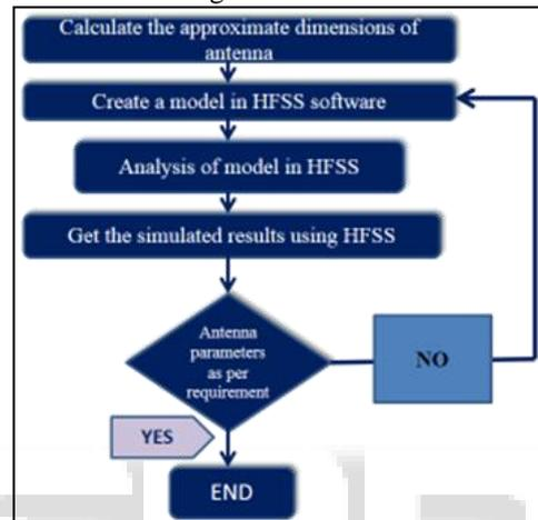
Fig. 7: Flowchart of Simulation
