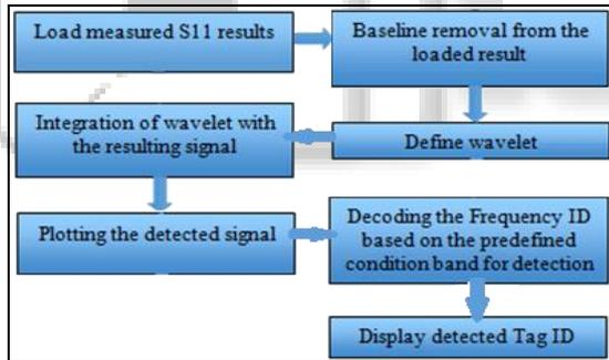
Fig. 8: Flowchart for Algorithm
