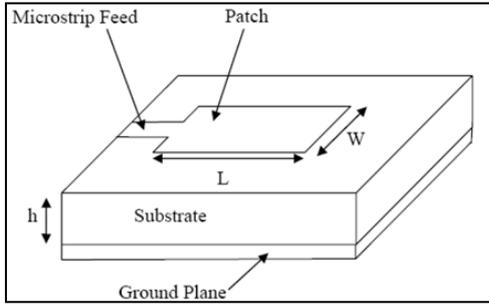
Fig. 5: Microstrip Antenna
