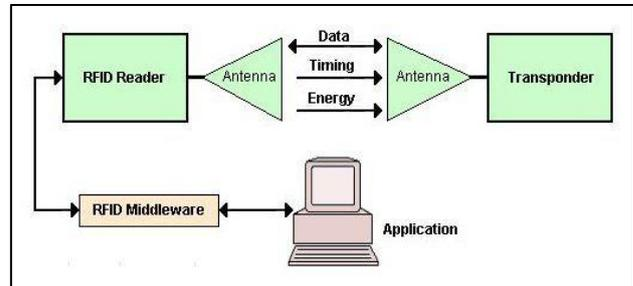
Fig. 1: RFID system components
