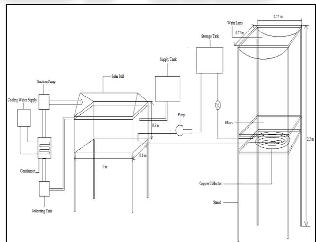
Fig. 1: Schematic diagram of solar distillation unit coupled with water lens concentrator
