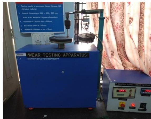
Fig. 1: Pin on Disk apparatus
