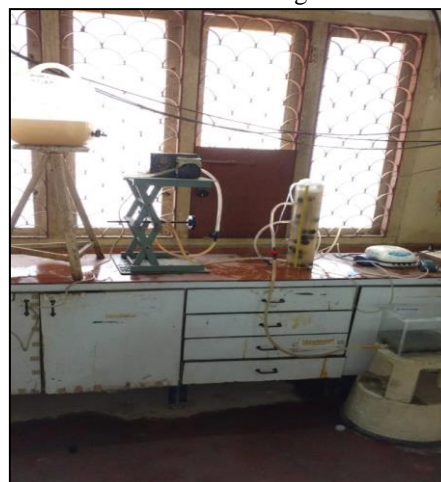
Fig. 4: Fabricated lab scale Fluidised Bed Biofilm Reactor
