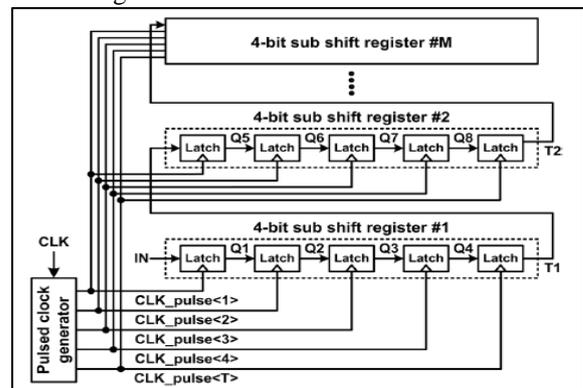
Fig. 7: Architecture of shift register
