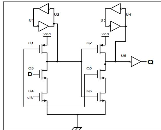
Fig. 1: Implicit pulsed Data Close to Out Flip-flop
