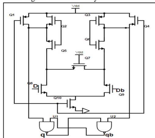
Fig. 2: sense amplifier flip-flop
