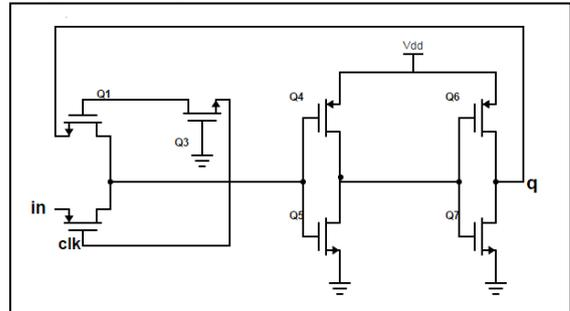
Fig. 6: Static Differential Sense Amp shared Pulsed Latch
