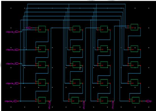
Fig. 10: Schematic of 16-bit shift register
