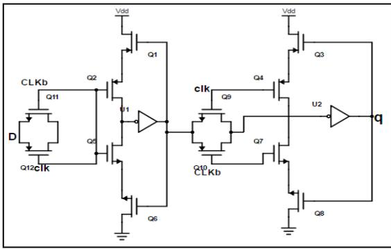
Fig. 3: Power PC Style Flip-Flop
