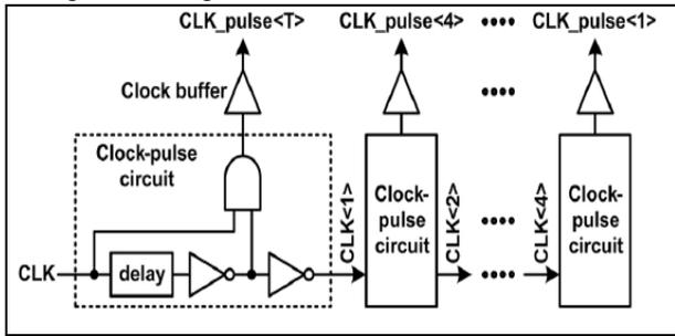
Fig. 9: Delayed pulse clock generator
