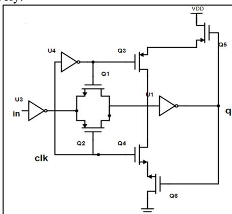
Fig. 5: Transmission Gate Pulsed Latch
