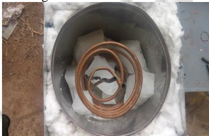
Fig. 2: Thermal Storage Inner Tank with Copper Tube
