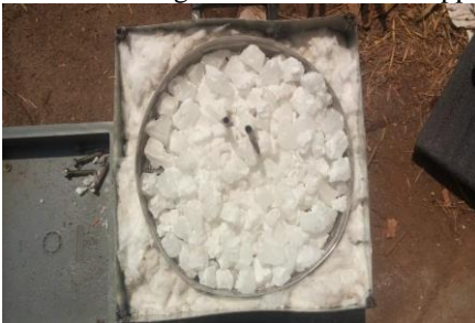
Fig. 3: Thermal Storage Tank with Paraffin Wax
