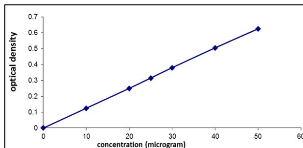
Fig. 2: Calibration curve for removal of  $Cr^{+6}$  using colourimeter
