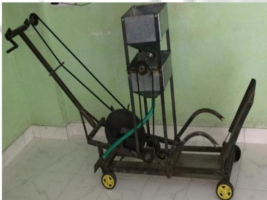
Fig. 1: Actual Model of Sowing and Planting Machine
