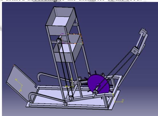
Fig. 2: CAD Model of Seed Sowing and Planting Machine
