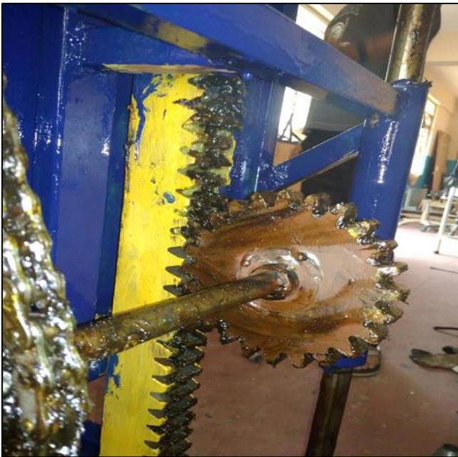
Fig. 5: Rack and pinion being used in present work.
