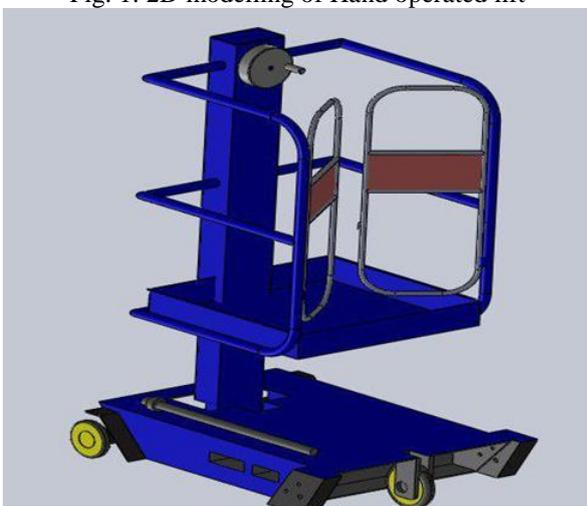
Fig. 2: 3D modelling of Hand operated lift
