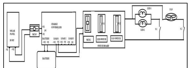
Fig. 6: Circuit Diagram of Solar DC Home System components of system
