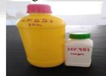
Fig. 11: Epoxy resin (LY556) &Hardener (951)
