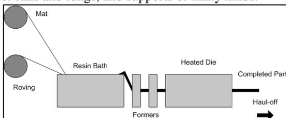
Fig. 3: Pultrusion Method
