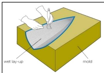
Fig. 1: Manual Lay-Up Technique Process Top view
