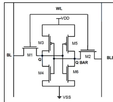
Fig. 1: Conventional 6T SRAM Cell
