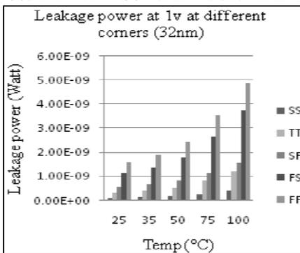
Fig. 5: Leakage power Vs Temperature variation at different process corner at 32nm
