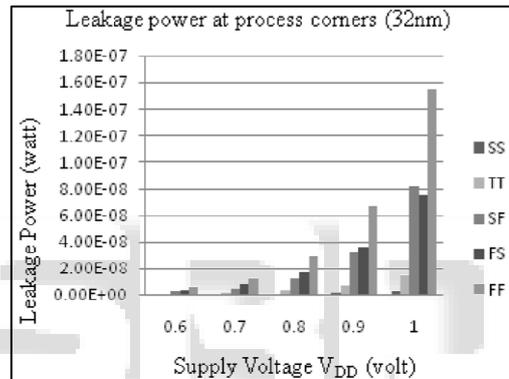
Fig. 3: Leakage power Vs voltage variation at different process corners at 32nm
