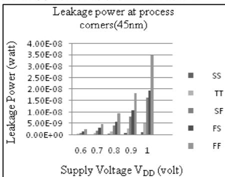
Fig. 2: Leakage Power Vs voltage variation at different process corners at 45nm.
