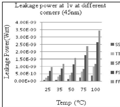
Fig. 4: Leakage power Vs Temperature variation at different process corner at 45nm
