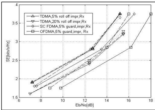
Fig. 2: Spectral efficiency vs. electrical SNR requirement of digital transmission schemes with an SSPA and AWGN in return link
