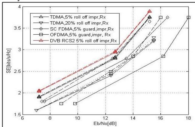
Fig. 3: Spectral efficiency vs. electrical SNR requirement of digital transmission schemes with an SSPA and AWGN in return link with DVB RCS2 transmission
